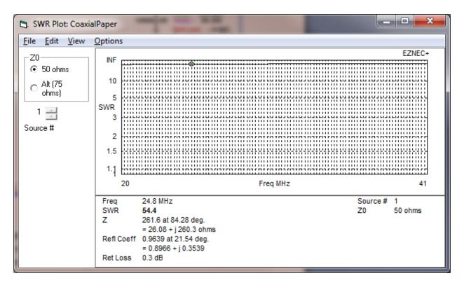
The above simulation shows the correct impedance at 24. Mhz. To get these results I had to set the coax los to 8db/100m.
