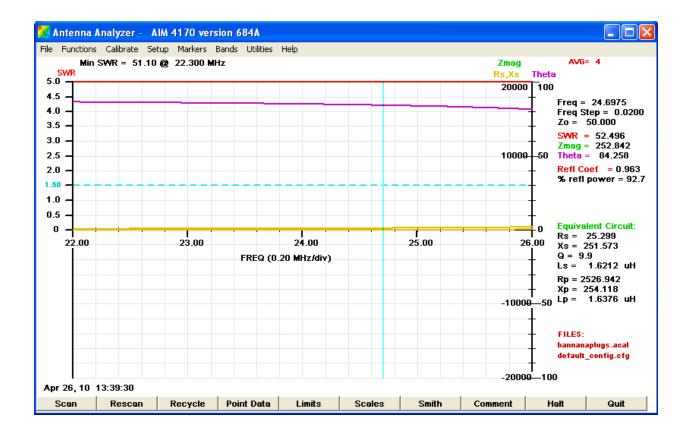
In the above scan I placed the cursor (vertical blue line) at the operating frequency. Notice the resistance is 25 ohms and the Q is only about 10. I knew the coax was cheap but this was way worse than I expected. I repeated my measurements in a variety of geometries and with multiple stubs. All were measurements were essentially the same. Using EZNEC I adjusted the coax loss to match the measured loss. Here is scan from EZNEC of just one of the coax segments:
