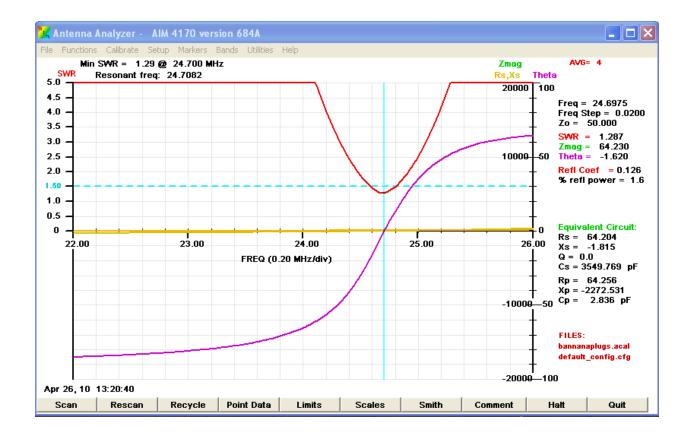
As can be seen from the above scan, EZNEC correctly predicted the resonant frequency. However, EZNEC did not correctly predict the impedance. EZNEC predicted 36 and I measured 64. This was unexpected and a little disconcerting so I went looking for an explanation.
