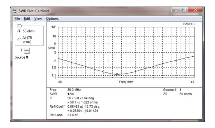
The first *measurement* I made was to find the natural frequency of the 'outer surface' of the coax. To make this measurement I connected my AIM 4170b antenna analyzer to the coax braid. I then lofted the antenna to 5 meters and ran a measurement. Here is the resulting scan:
