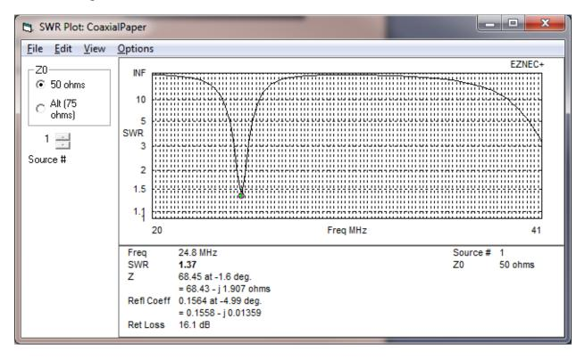
This matches VERY NICELY with the actual measurements. From these measurements and simulation I conclude that the coaxial cable operates along the lines predicted by the simplified model.
