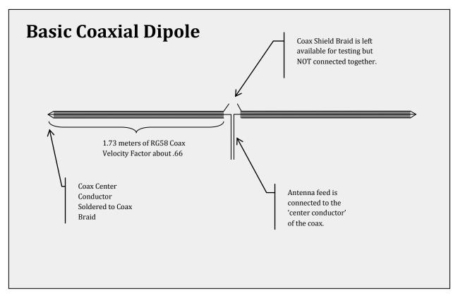
This antenna has much in common with the 'double bazooka' and my immediate 'gut feeling' was that the coax performs two functions. First, the radiating elements of the antenna would be the outer surface of the coax shield. Second, the coax segments would provide some reactance, presumably inductive, which would lower the resonant frequency of the basic dipole. In order to simplify thinking about these two functions I redraw the antenna as:
