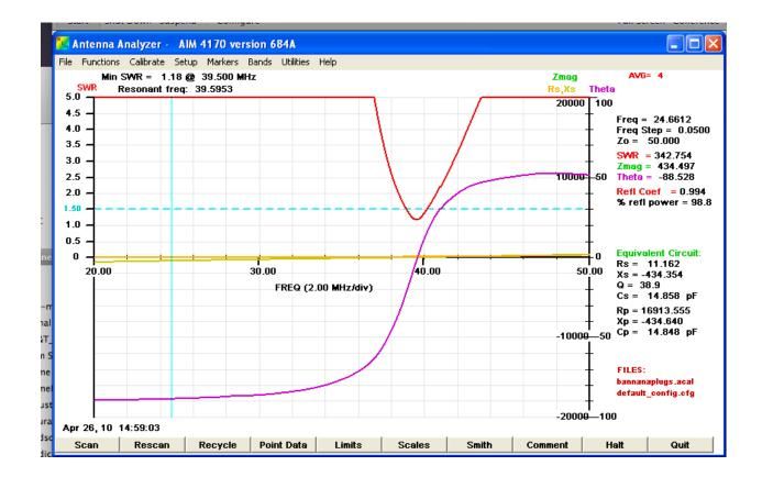
As can be seen in the trace, the coax 'braid' resonated at about 39.5 MHz. I made the same measurement after connecting the center conductors and the braids at both ends. The scan was unchanged. Thus, EZNEC simulation and actual measurement matched up surprisingly well. Thus, we can be reasonably certain that we understand the 'radiating' piece of the antenna.
