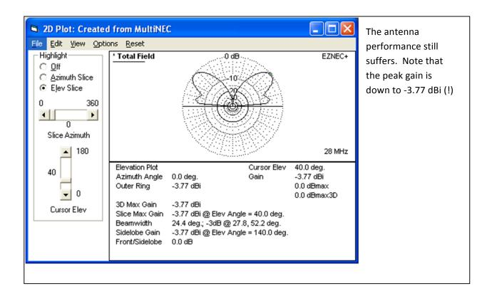
As has been shown the 'rule of thumb', 500 ohm chokes are inadequate to suppress feed line currents in these antennas. What happens when the choke impedances are increased to the 2800 ohm level:
