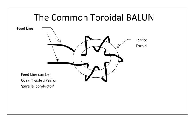
This type of choke has many advantages. Its construction is relatively simple and tolerant of variation. It is useful over very wide bandwidth; usually more than a decade. And it is relatively small and lightweight.
