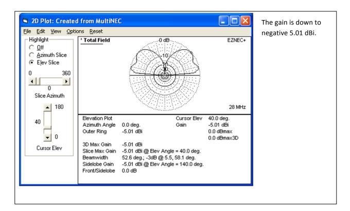
Earlier sections suggested that a second choke can be added to help with feed line currents. However, it has already been shown that low value chokes placed at low current points have little effect. Here is a plot of the currents with TWO 500 ohm chokes installed as previously described:
