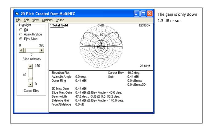
Finally, it is possible that only one choke need be 'good'. What happens if the choke at the top of the feed line (bottom of the dipole) is 7800 ohms but the choke in the middle is only 500:
