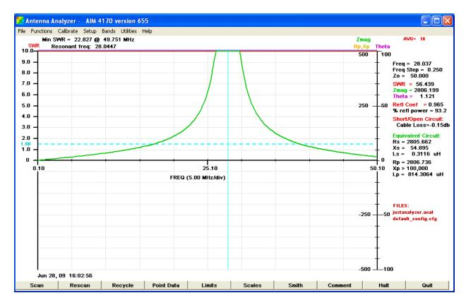
The above plot shows that the RG58U was resonant at 28.04 MHz and that the impedance was about 2800 ohms at this frequency. Importantly, the impedance was not INFINITE which means that the RG58U coax was lossy.
