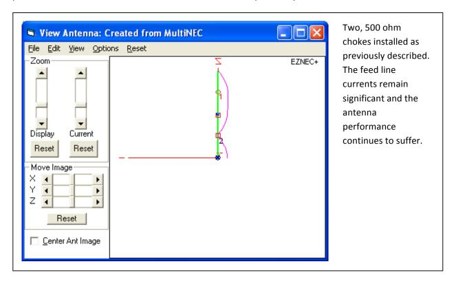
As can be seen above and as expected, the second choke provides no real improvement. The next step would be to add a third choke:
