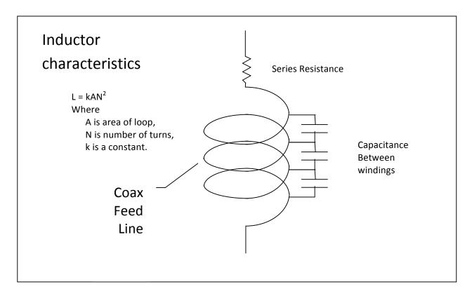
The imperfections of inductors derive from their very construction. Inductors must be made from real conductors which have real resistance. In addition, because the coax is coiled there will be some capacitance between neighboring windings. Generally, chokes should be constructed using nice, neat winding techniques rather than a bunched together. This is largely because the results are more predictable and reproducible.
