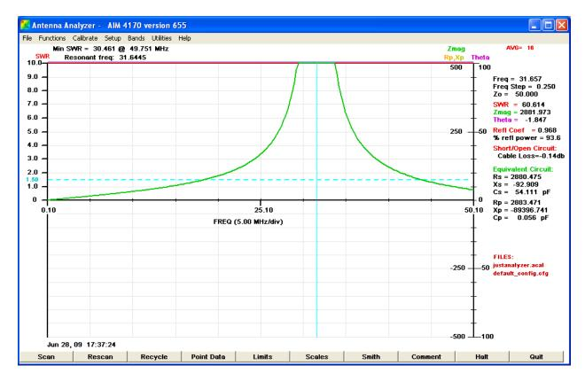
The resonant frequency is now higher, up to 31 MHz. because the insulating material is now air. More importantly, the impedance has gone back up to 2880 ohms; higher than the RG58U itself. Thus, the losses and length of the sleeve choke are controlled by the insulating material between the coax shield and the sleeve conductor.
