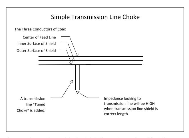
The next step is to turn the transmission line choke 90 degrees. The two surfaces of the added transmission line are shown here as collapsed:
