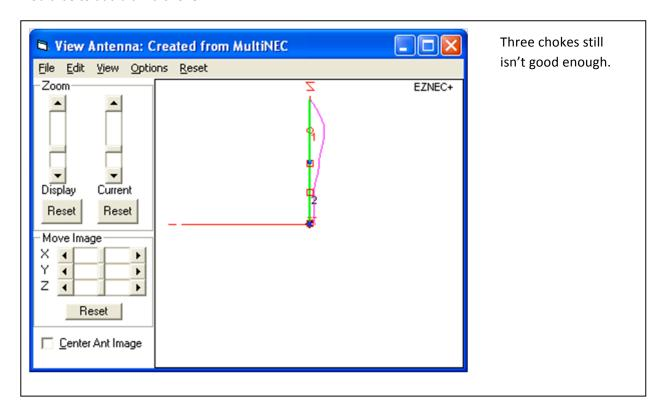
It is clear at this point that 500 ohm chokes will not be sufficient to control the feed line currents of the COAXIAL/BAZOOKA/RFL antennas in all situations. This may well explain why casual construction of this class of antenna often results in poor performance. Since 500 ohm chokes are insufficient, the next question is, what impedance is required. The following what happens as the impedance is increased:
