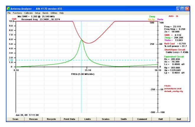
Note the resonant frequency is now 23.3 MHz. If the length of the sleeve was dictated by the velocity factor of the coax then the frequency would be unchanged. Since the frequency did change the only conclusion is that the coax jacket, rather than the internal dielectric, must determine the sleeve velocity factor.
