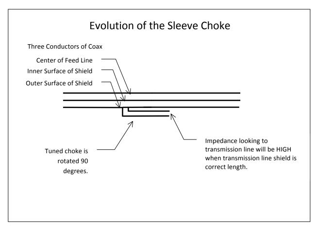
The last step is to join the outer surface of the coax shield and the close part of the transmission line choke:
