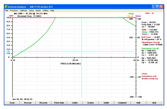
Casual examination of the above graph shows that these coils can be effective over very wide frequency ranges. Above, an impedance of 500 ohms is provided from about 17 MHz up to about 45 MHz; almost a factor of 3.
