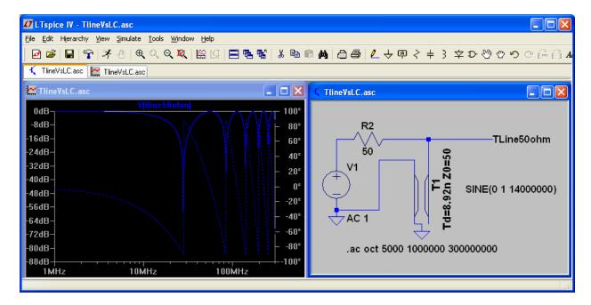
Thus, a simple piece of transmission line such as coax can be used to implement an inductor, a capacitor and even an LC circuit. This flexibility, when integrated with feed lines, can be exploited to implement tuned chokes.
