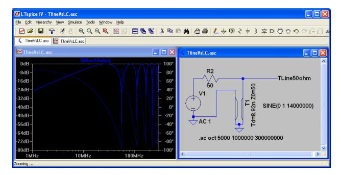
A few observations of the simulation are in order. To start, the transmission line has a propagation of 8.92 ns. which corresponds to a design frequency of 28 MHz. The left side of the graph is a relatively low frequency. Here, the transmission line is acting much like an inductor; increasing frequency results in an increasing impedance.
