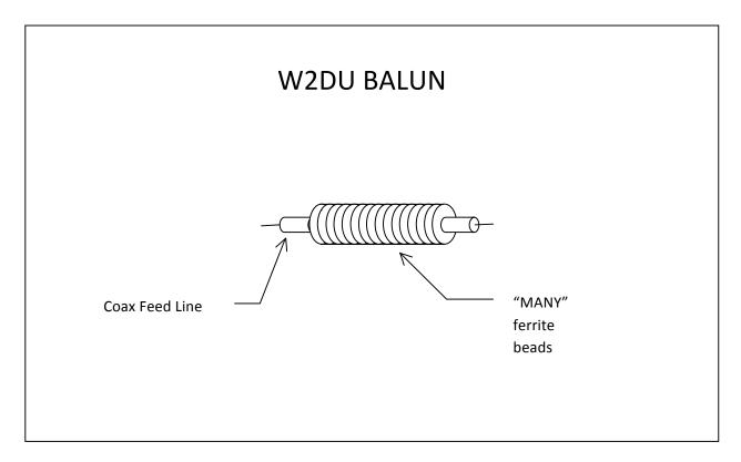
The inductance of the W2DU BALUN is essentially proportional to the number and type of ferrite beads used. The beads need not be all the same and so the W2DU BALUN can be designed to cover extremely wide bandwidths.
