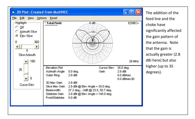
Previous writings have indicated that a feed line choke added at a feed line current maximum would help. That choke is now added:
